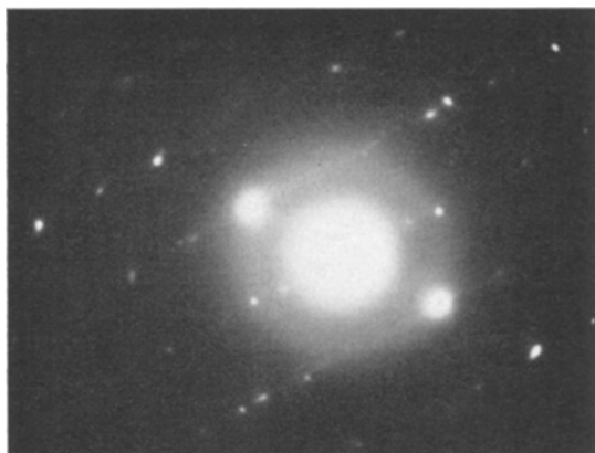
Figure 3 Selected-area electron diffraction pattern of region shown in fig. 2.
